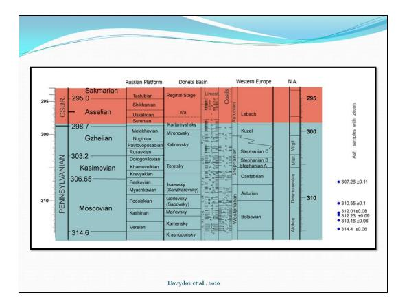
New radiometric data provided highly precise framework for the detailed lithostratigraphic, biostratigraphic, and cyclostratigraphic research. In construction of our cyclicity model we use material from four sections in the interval of the Podolskian, Myachkovian, and Kasimovian in the Donets Basin, as well as published data from the Eastern European Platform, Southern Urals, Central Asia, Cantabrian Mountains and China.
