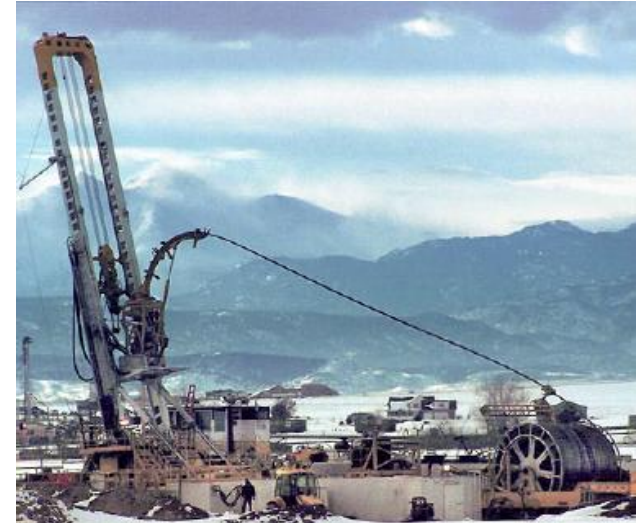
Anadarko Petroleum began using a coiled tube rig in November in the Wattenberg oil and gas field in eastern Colorado. The newer rigs are smaller and more portable than standard rigs. (Special)
