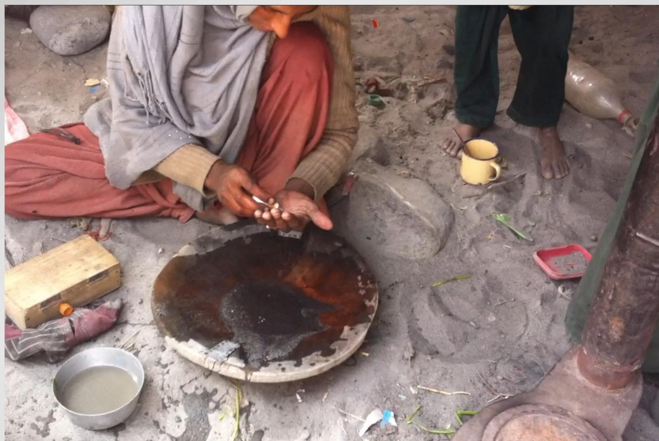
Figure 5. A photo taken during field trip. The lady in the picture is putting some drops of liquid mercury to amalgamate panned sediments from Hunza River. After being mixed with the sediment, mercury is let to evaporate by heating in the stoves it their tents (seen on right side) to recover gold. Notice that no health risks are considered in the amalgamation and roasting processes.
