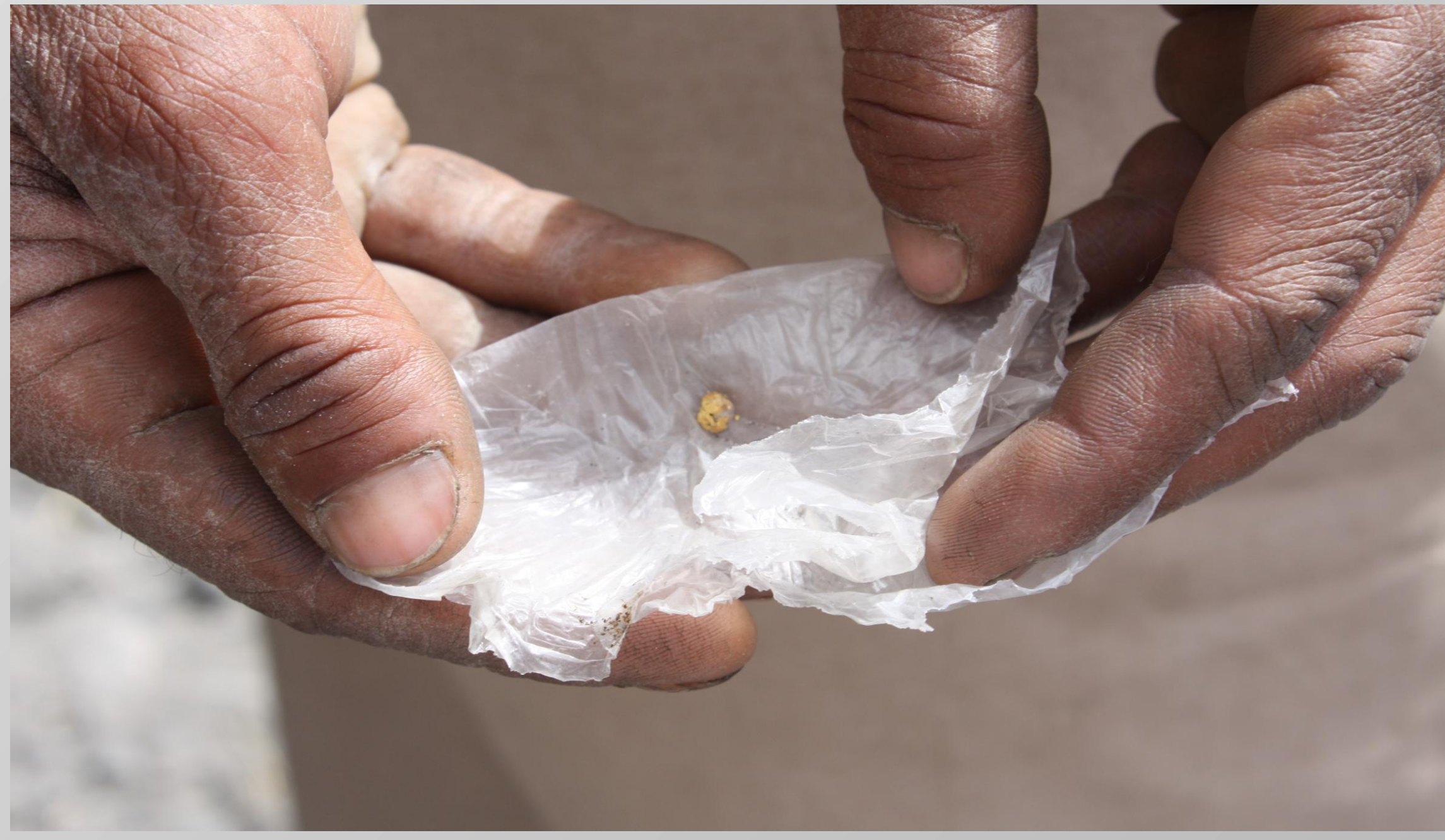
Figure 6. Photo showing the recovered gold after evaporation /roasting process. The raw gold is further refined by gold-dealers and goldsmiths in shops and refinement places. This small-scale GPE process is similar in all selected sites of the study area.
