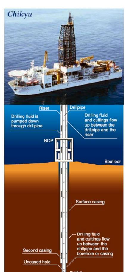
Why & How it was Drilled The cores that were recovered from Site C0001 & Site C0002 during the Integrated Ocean Drilling Project (IODP) Expedition 315 in the Nankai rough, by the Chikyu Hakken. These cores were recovered as part of the Japanese-led initiative to drill through the Eurasian Plate - Philippine Sea Plate interface, as well as answer fundamental questions about subduction zone margins.
