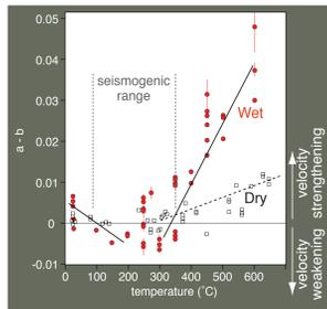
Figure 1. Results of laboratory experiments on wet and dry granite samples. a-b represents the change in friction upon increasing sliding velocity. If negative, it indicates velocity-weakening behavior, where initiated slip is likely to continue and result in an earthquake. If positive, it indicates velocity strengthening, where friction increases and slip ceases. The 'seismogenic range' falls in the temperatures of velocity weakening behavior. Modified from Blanpied et al., 1995.
