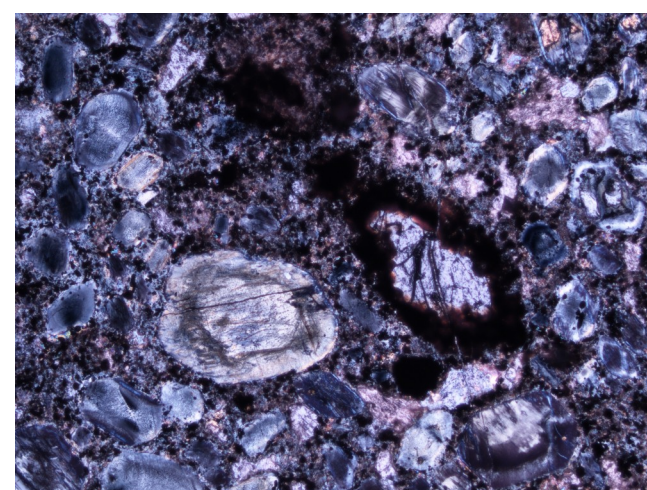
Sample 1, Ilmenite Banding, 40x
