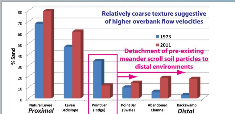
Figure 7. Average % sand content of overbank sediments deposited by the 1973 (Kesel *et al.*, 1974) and 2011 Lower Mississippi River floods in various depositional sub-environments in the study area.
