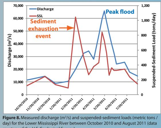
Figure 8. Measured discharge (m<sup>3</sup>/s) and suspended-sediment loads (metric tons / day) for the Lower Mississippi River between October 2010 and August 2011 (data courtesy of the U.S. Geological Survey).
