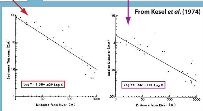
Figure 11. Sediment thickness (cm) and median particle size (mm) of overbank sediments deposited by the 1973 Lower Mississippi River flood in the study area (Kesel *et al.*, 1973). A cursory comparison with the 2011 data above (Figures 9 and 10) indicates better defined trends with distance from the river channel in 1973.
