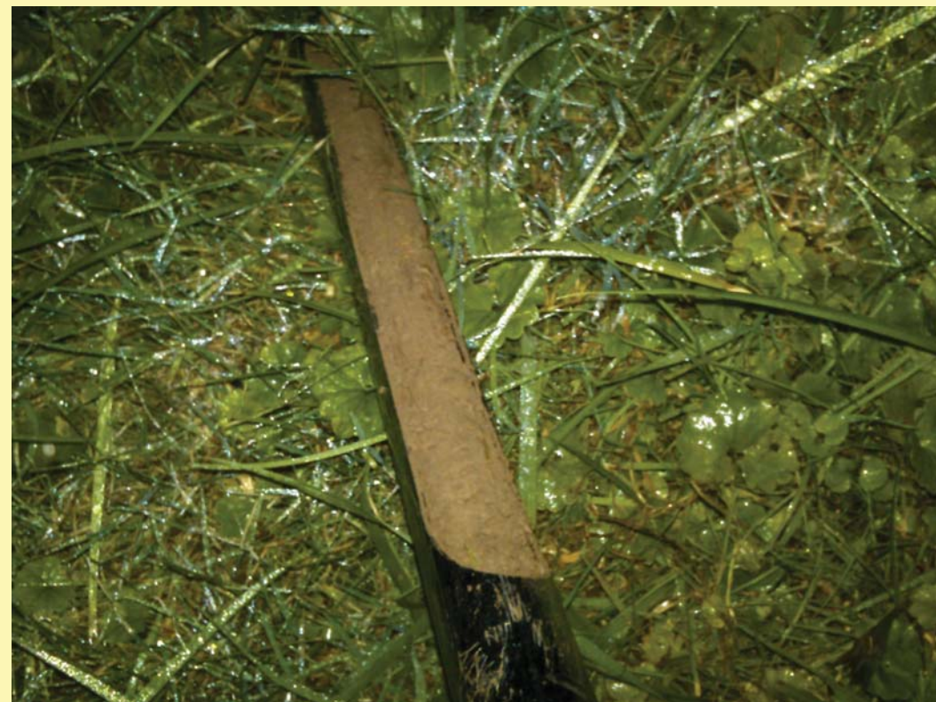
Figure 15. Soil core gravimetric and volumetric analysis was used as a direct measurement to estimate SWC. 2 cm diameter soil cores were taken 2 meters southeast of the GPR CMP. The cores were individually bagged, weighed, and dried in an oven at 60 degrees celcius for two weeks. They were then reweighed and SWC was calculated.
