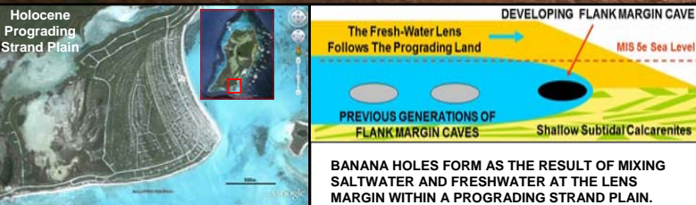
Figure 3: The new model explains the great abundance of banana holes in the Bahamas, and their relative absence in reef-limestone islands. It also explains their small size and simplicity as immature flank margin caves, and requires no problematic vadose/phreatic fresh-water mixing geochemistry.
