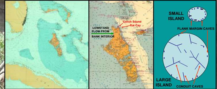
Figure 4: During glaciations, eustatic sea-level fall changes small islands into big islands. Meteoric catchment area increases by the square, but the discharge perimeter increases only linearly. This input/output imbalance leads to the development of conduit caves as well as flank margin caves.
