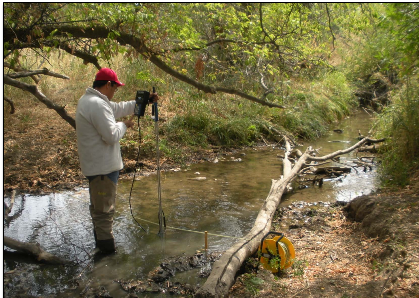
Sampling a tributary of the Little Bighorn River for metals and measuring flow, part of the Crow Water Quality Project
