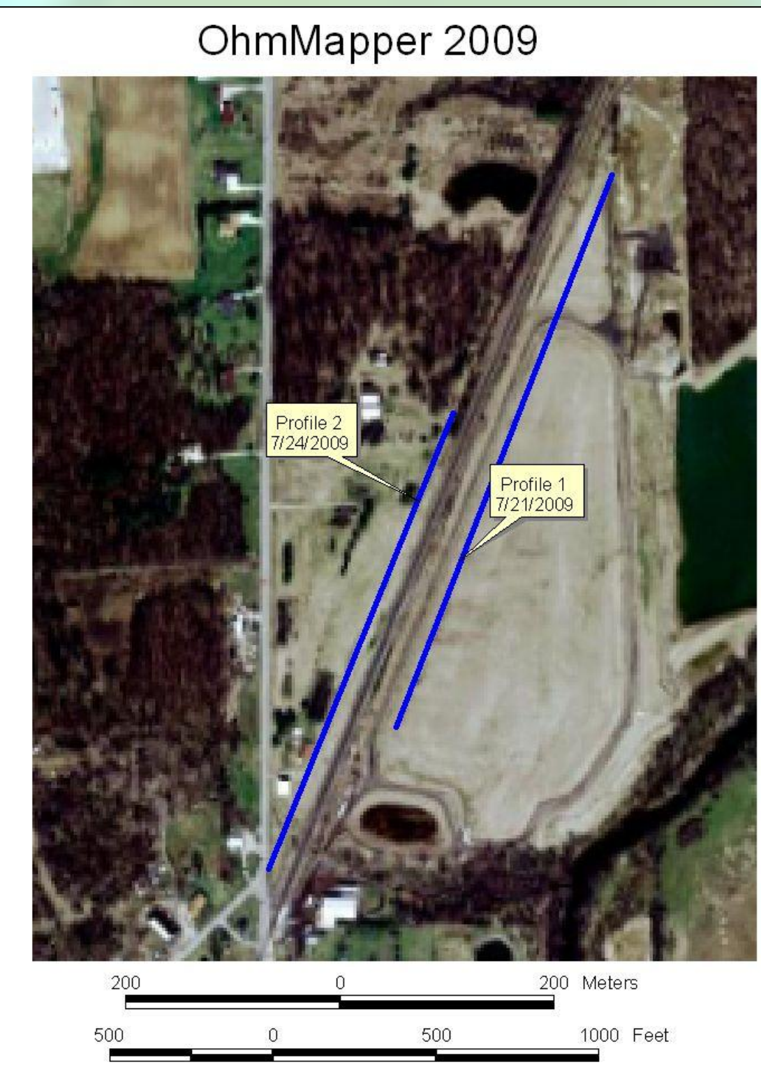
Figure 6: aerial image of landfill and OhmMapper profiles.
