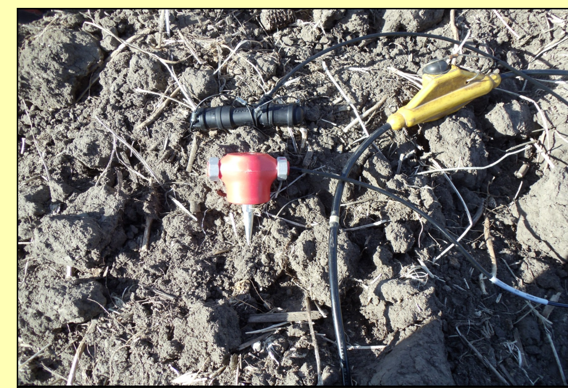
Low Frequency Geophone (4.5 Hz)
