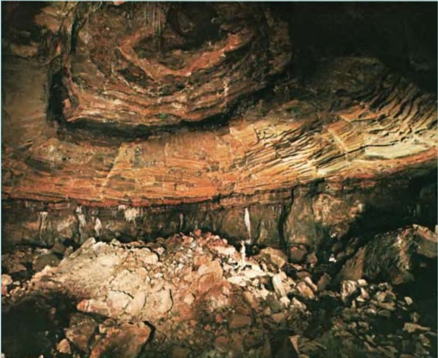
Cavity produced by Gnome detonation and subsequent collapse 70 feet high and >150' across (miner at right center of rubble pile). Photo by Lawrence Radiation Laboratory
