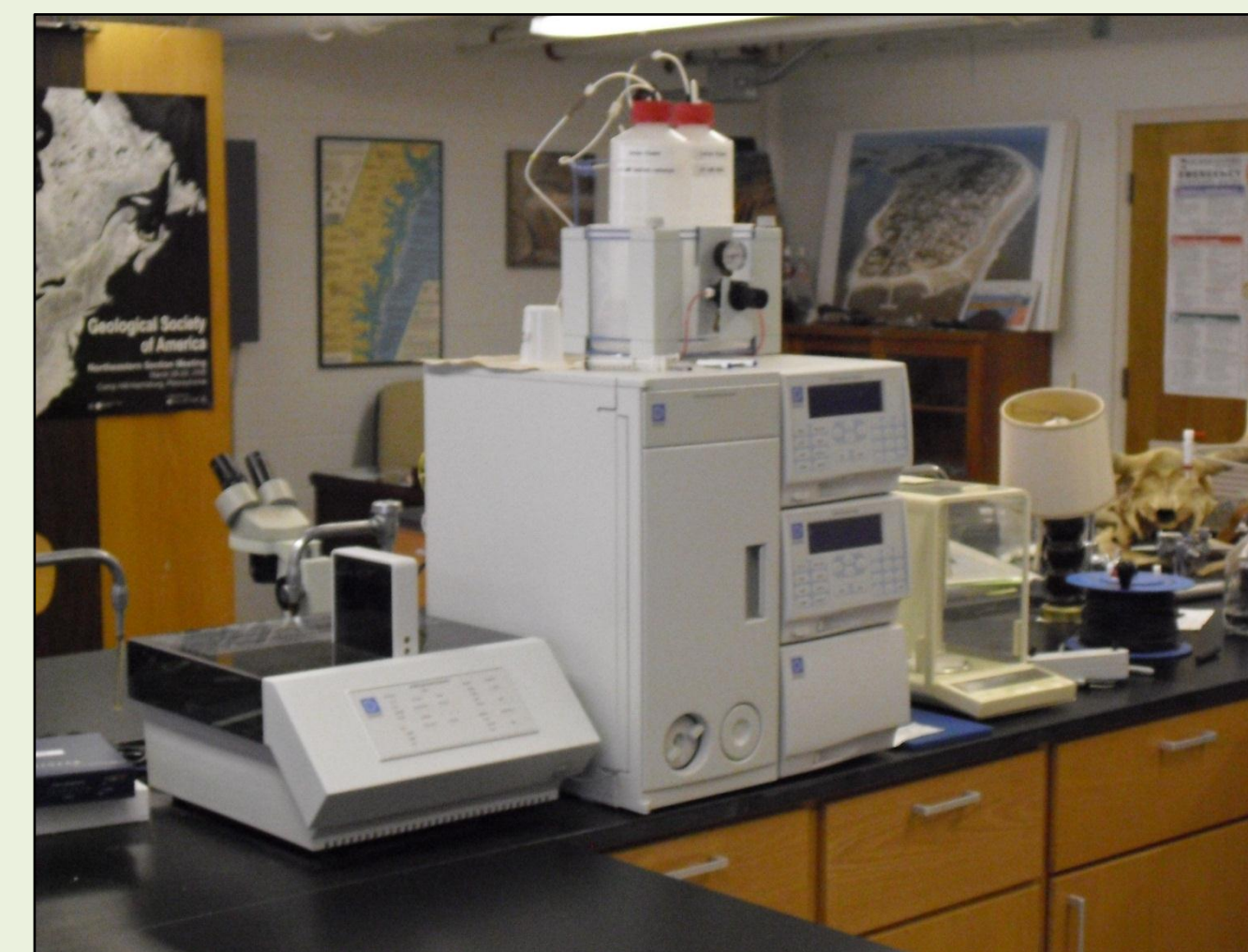
Figure 4. Ion chromatograph in GSU hydrogeochemistry lab.
