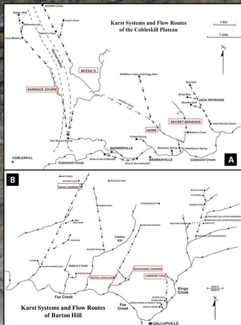
**Figure 2:** A: Map of the karst systems and flow routes of the Cobleskill Plateau. The buried valley is located between Barrack Zourie Cave and McFail's Cave (re-drawn from Dumont, 1995). B: Map of the karst systems and flow routes of Barton Hill (re-drawn from Mylroie, 1977). Red boxes denote caves investigated by this study.
