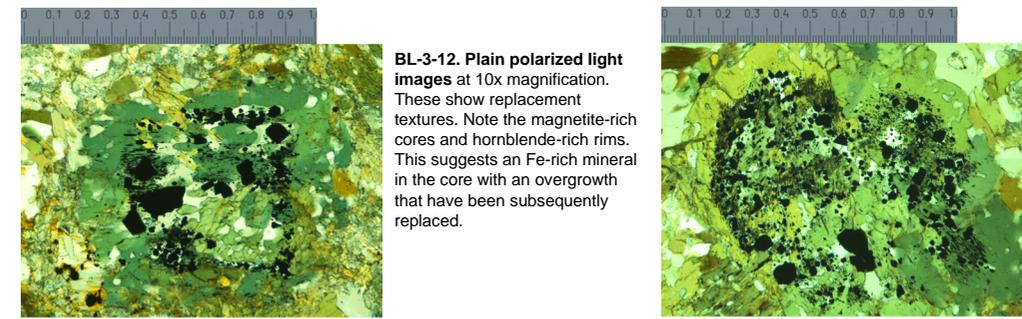
BL-3-12. Plain polarized light images at 10x magnification. These show replacement textures. Note the magnetite-rich cores and hornblende-rich rims. This suggests an Fe-rich mineral in the core with an overgrowth that have been subsequently replaced.
