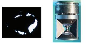
Fe<sub>2</sub>O<sub>3</sub> powder is loaded into a panoramic DAC with Be gasket, with He or Ne as pressure transmitting medium.
