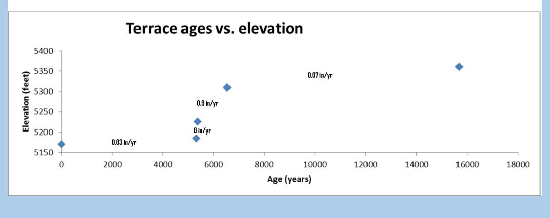
The North Platte River has been degrading its channel over a period of at least 15,000 years in the Casper area. This erosion has been punctuated by at least two periods of stability (slow erosion rate) and one episode of swifter incision.
