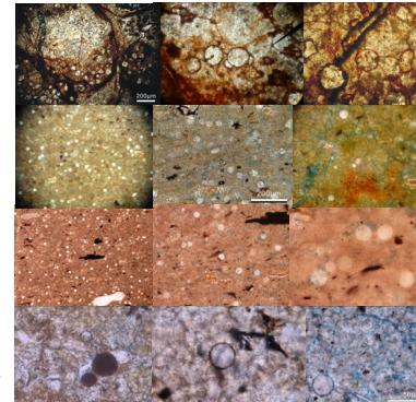
Dolomite, micron-sized spheroids (6-20  $\mu$ m), and shell fossil fragments in petrographic thin sections
