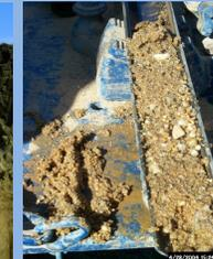
Figure 3 Split Spoon Sample Displaying Stratified Drift
