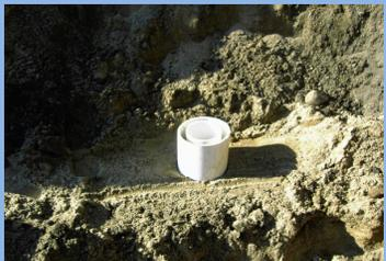
Figure 4 Conducting Infiltration Test
