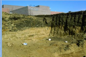
Figure 2 Test Pit Showing Dark Gray, Organic-rich Topsoil Capping Stratified Drift
