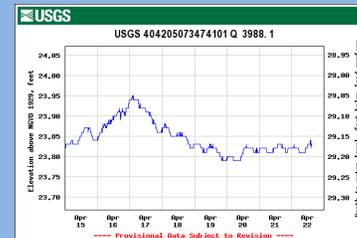
Figure 8 A Typical Groundwater Table Recording of York College Monitoring Well (USGS)
