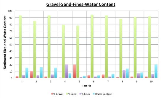
Figure 9 Textural and Water Content Data Involving Test Pits and York Monitoring Well (Sample #10)
