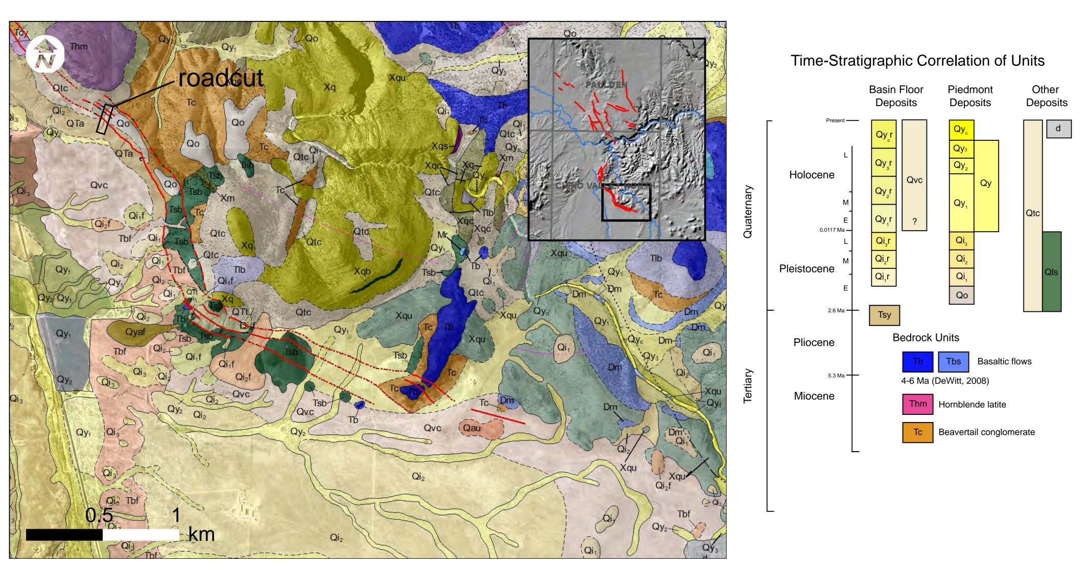
Geologic map superimposed over the same area shown to left, emphasizing Quaternary units in relation to faulting. Legend of mapping units and relative ages to right.
