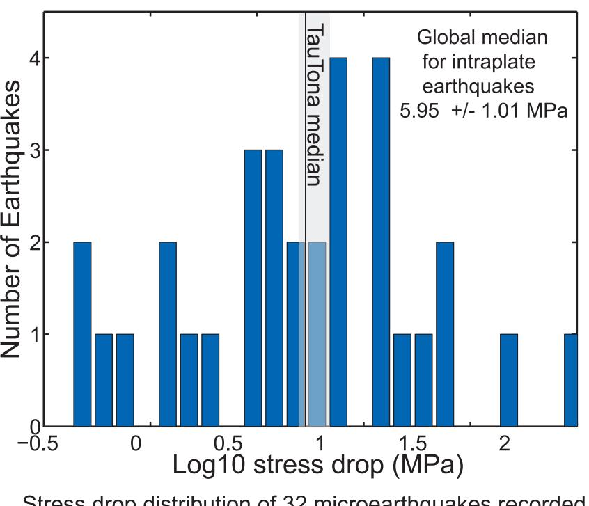
Stress drop distribution of 32 microearthquakes recorded at TauTona Gold Mine (global median from Allmann and Shearer, 2009)
