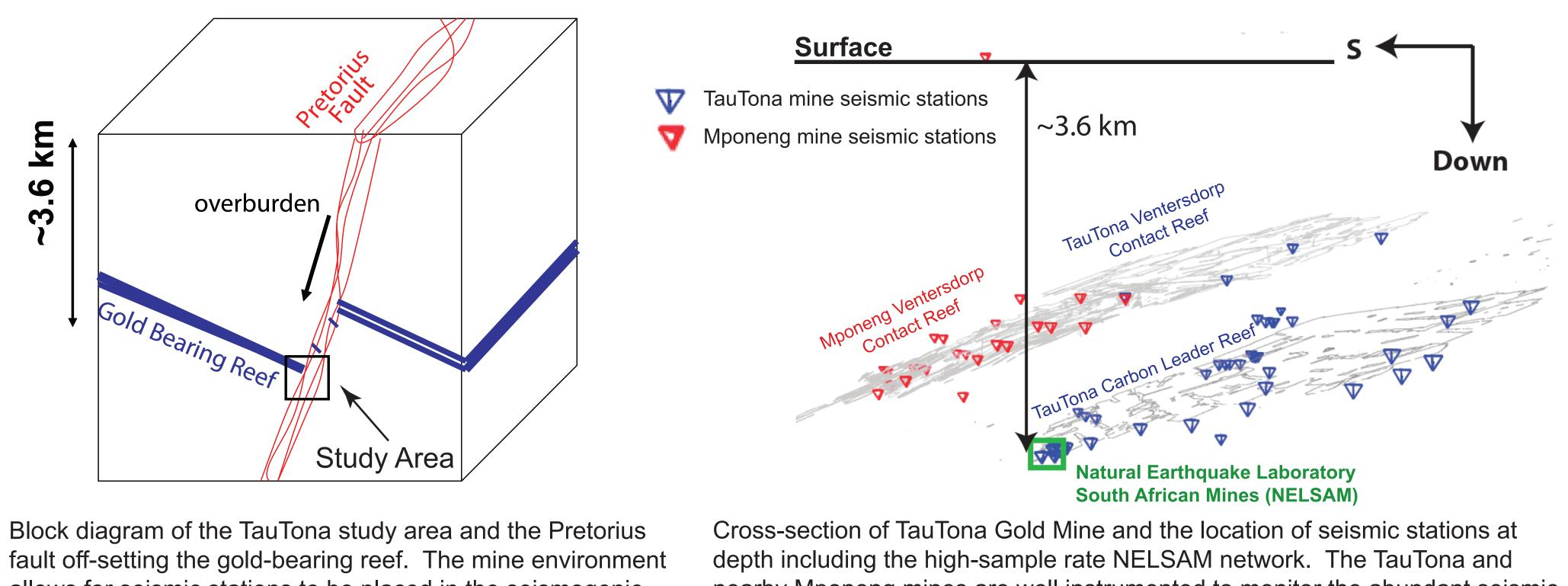
Block diagram of the TauTona study area and the Pretorius allows for seismic stations to be placed in the seismogenic zone next to hundreds of earthquakes that occur everyday.
