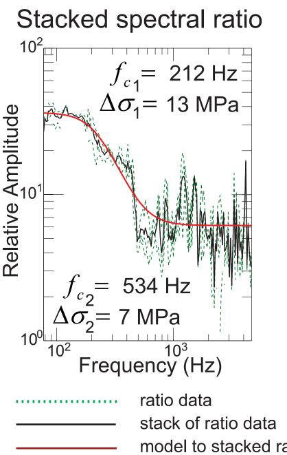
The spectral ratios for each component and station are stacked and modeled to find the corner frequency
