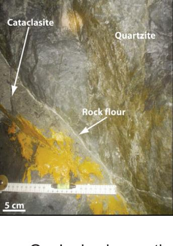
Geologic observations of a subparallel segment of the Pretorius fault that slipped after a M2.2 earthquake on 12 December, 2004.
