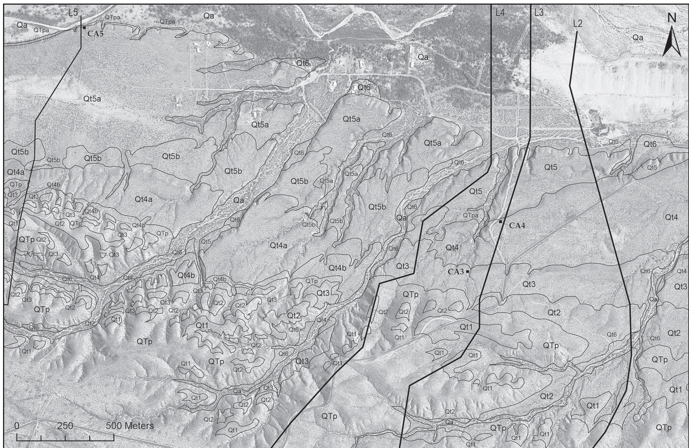
FIGURE 6. Map of Cañada Alamosa terraces (Qt map units) developed in the Palomas Formation (map unit QTp) or in its axial Rio Grande facies (QTpa) of study area 1. Locations of soil profiles CA3-5 and topographic profiles L2-L5 are shown. Note how terraces Qt4b and Qt5b step down from the west to form a single lower terrace surface to the east of the drainage immediately left of profile L4.
