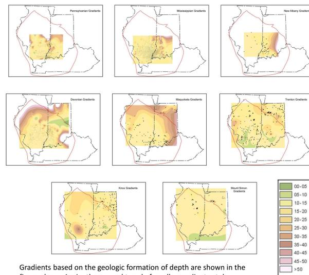
Gradients based on the geologic formation of depth are shown in the figure above. Again, the general trend of smaller gradients at deeper depths can be seen.
