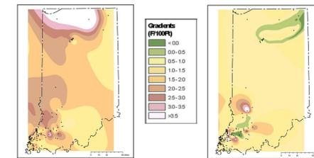
Wells that had two depths and temperatures recorded on geophysical logs. The figure on the left is an interpretation map of the geothermal gradients for the shallow portion of the wells while the figure on the right is the gradients for the deeper section of the well.
