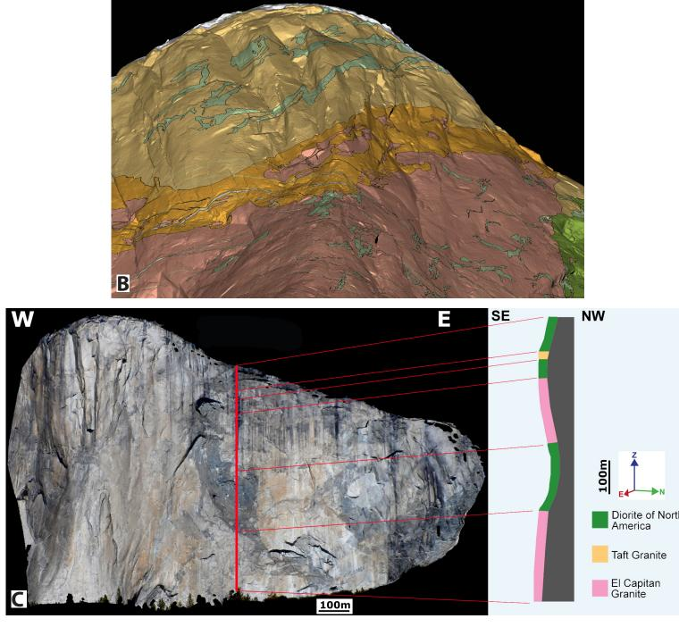
Using Reshaper 3D<sup>tm</sup>, the geologic map was overlain over terrestrial lidar scans of El Capitan. This gave a general picture of the slope in areas occupied by different rock types. Several correlations are evident:
