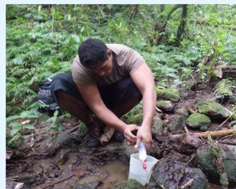
Figure 4: Radon grab samples were taken with a gas tight piezometer and hand-pump to minimize dissolved gas evasion. Samples were analyzed on a RAD 200 radon gas detector the same day as collection.
