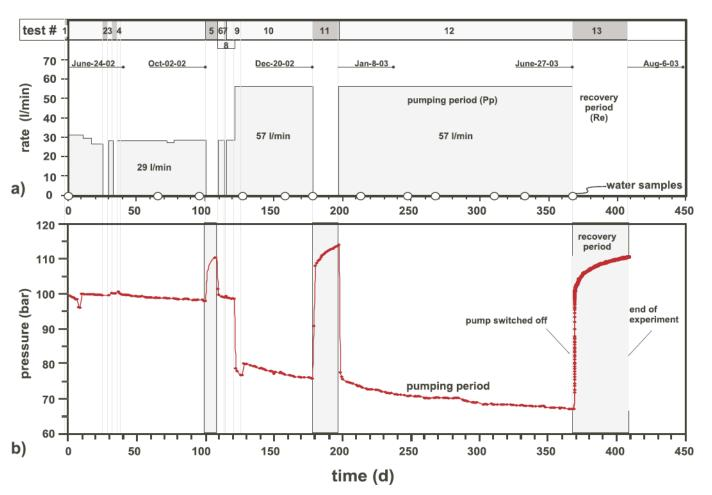
Long-lasting pumping-tests, KTB-site, 4 km depth:
