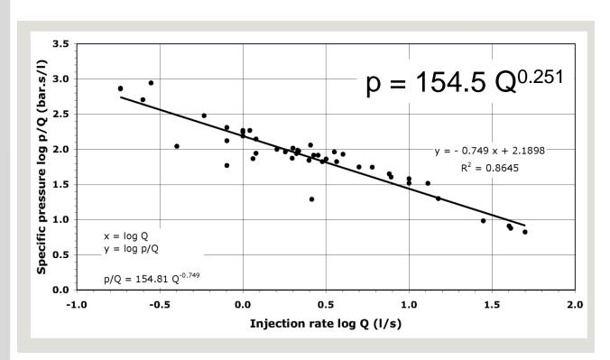
Elastic reaction of the rock: fractures are widened
