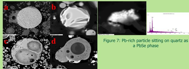
Figure 6: The 3 major types of glasses on fly ash particles by EMP analysis [(a) Fe-rich, (b) Ca-rich and (c) AlSi-rich] and (d) Fe concentrated on AlSi fly ash particle's surface
