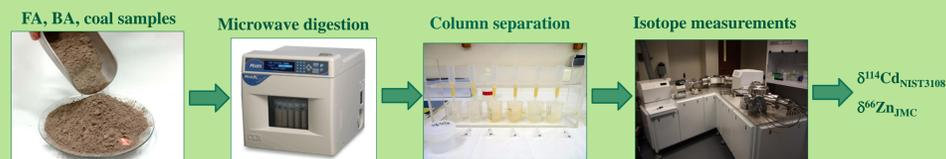
Figure 2: Analytical procedure for Cd and Zn isotopic measurements for CCP samples
