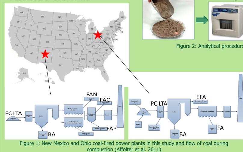
Figure 1: New Mexico and Ohio coal-fired power plants in this study and flow of coal during combustion (Affolter et al. 2011)
