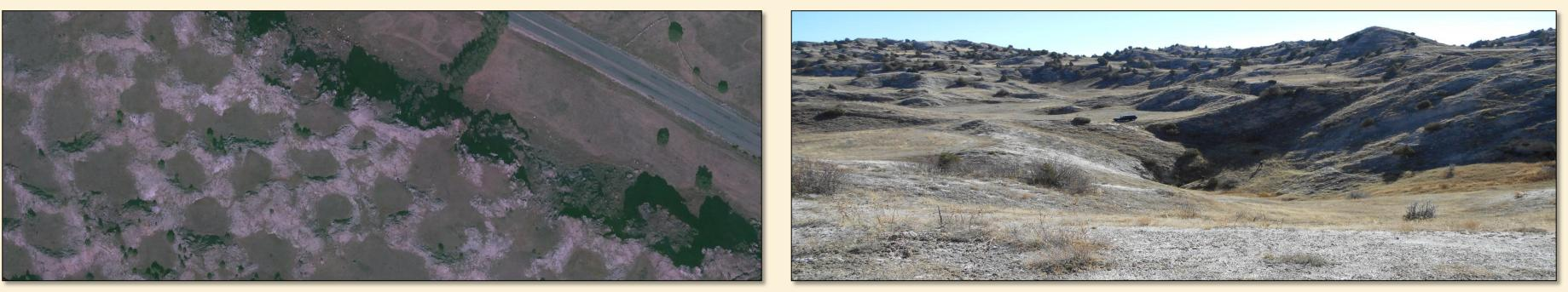
**ENGINEERING RECOMMENDATIONS:** Locally re-route pipeline to follow bedrock exposures and minimize crossing identified sinkholes. Implement surface drainage controls to minimize sinkhole evolution. Minimize pipeline length along karst margins. Install thicker pipe capable of 30-m free spans in area of plateau karst area (20 km).
