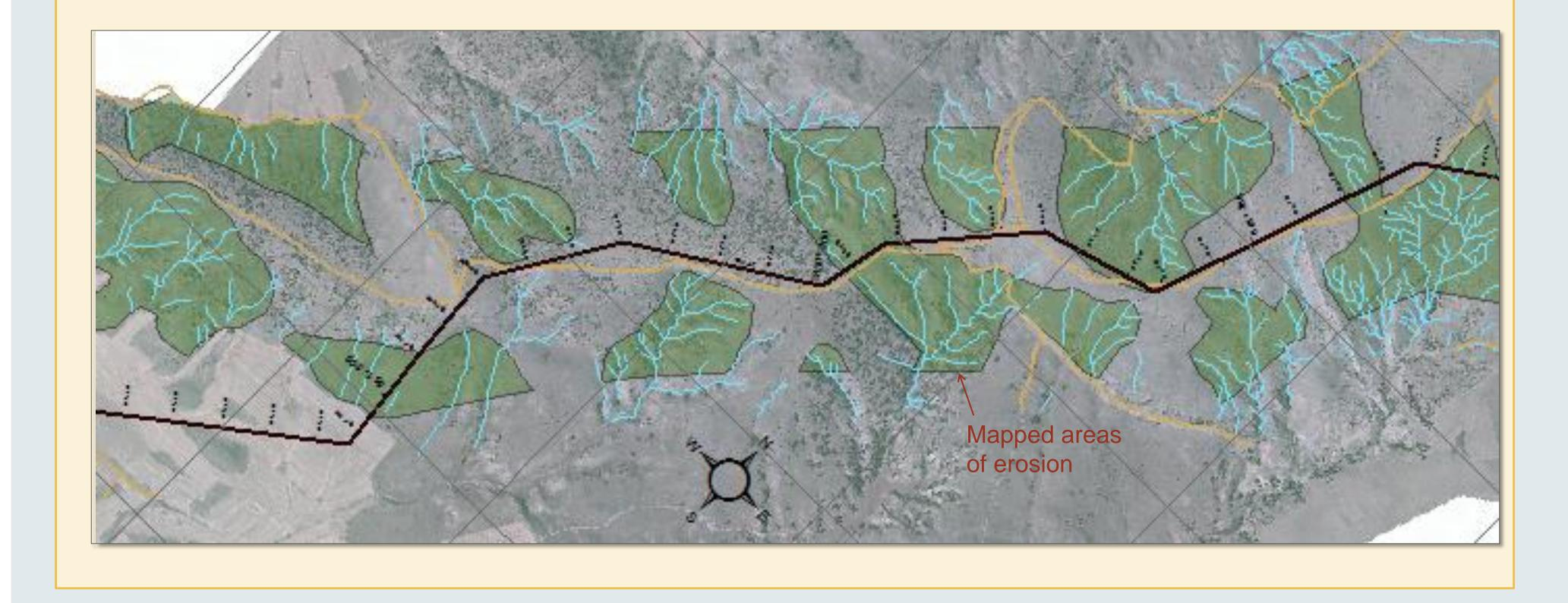
**ENGINEERING RECOMMENDATIONS:** Install pipeline tie-downs/anchors in zones susceptible to liquefaction to resist uplift. Locally re-route to eliminate lengths adjacent and parallel to a free face (e.g., river bank). Include deeper burial below zones of potential lateral spreading.
