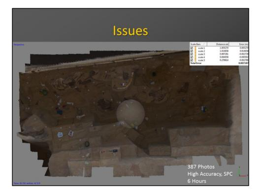
Camera was farther away so the model has less detail when zoomed in and more error across the model area. Also issues with shadows and there is the need for oblique photos of the area to aid in texture generation for side areas (like the walls).
