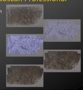
Can build a sparse point cloud or a dense point cloud – has potential to have more data points than a laser scanner.
