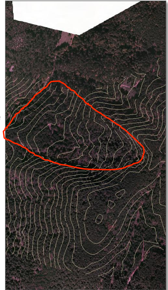
Aerial imagery with topography with landslide feature
