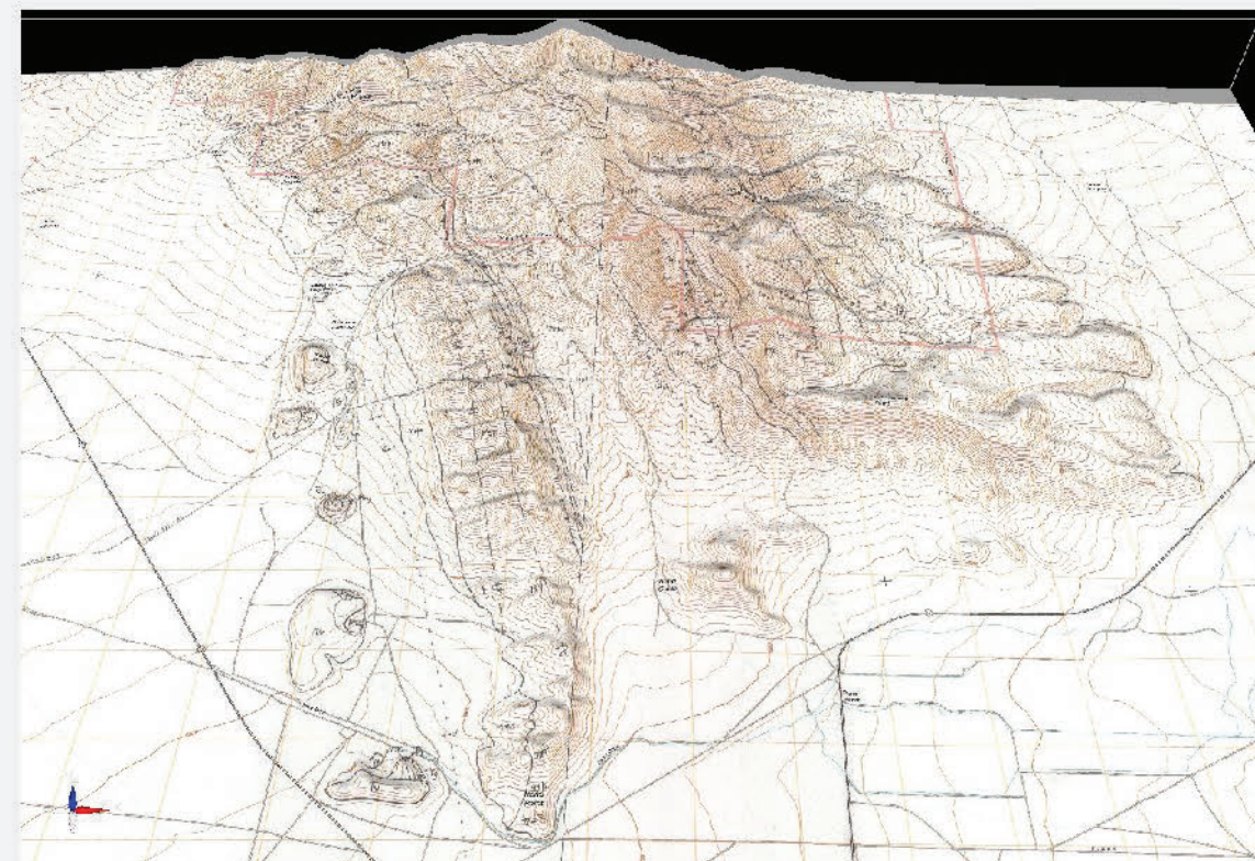
First step is to georegister the geologic maps, shown here draped on the topography in earthVision software.
