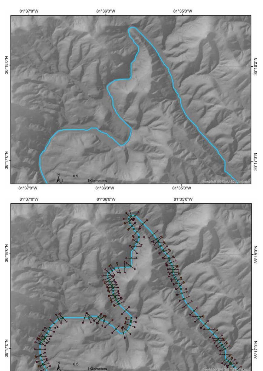
We located channels of interest using a USGS streams and rivers shapefile, and created representative polylines using the cost path tool available in ArcMap.
