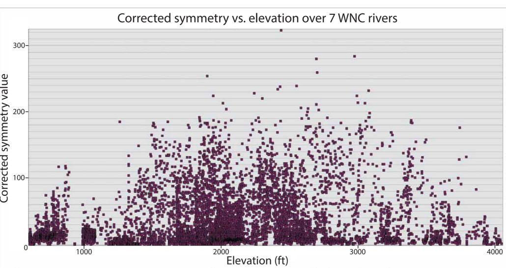
This figure illustrates the relationship between altitude and corrected symmetry. Maximum corrected symmetry values are visible between 1500-3400 ft, indicating that streams at intermediate elevations experience minimal lateral migration.
