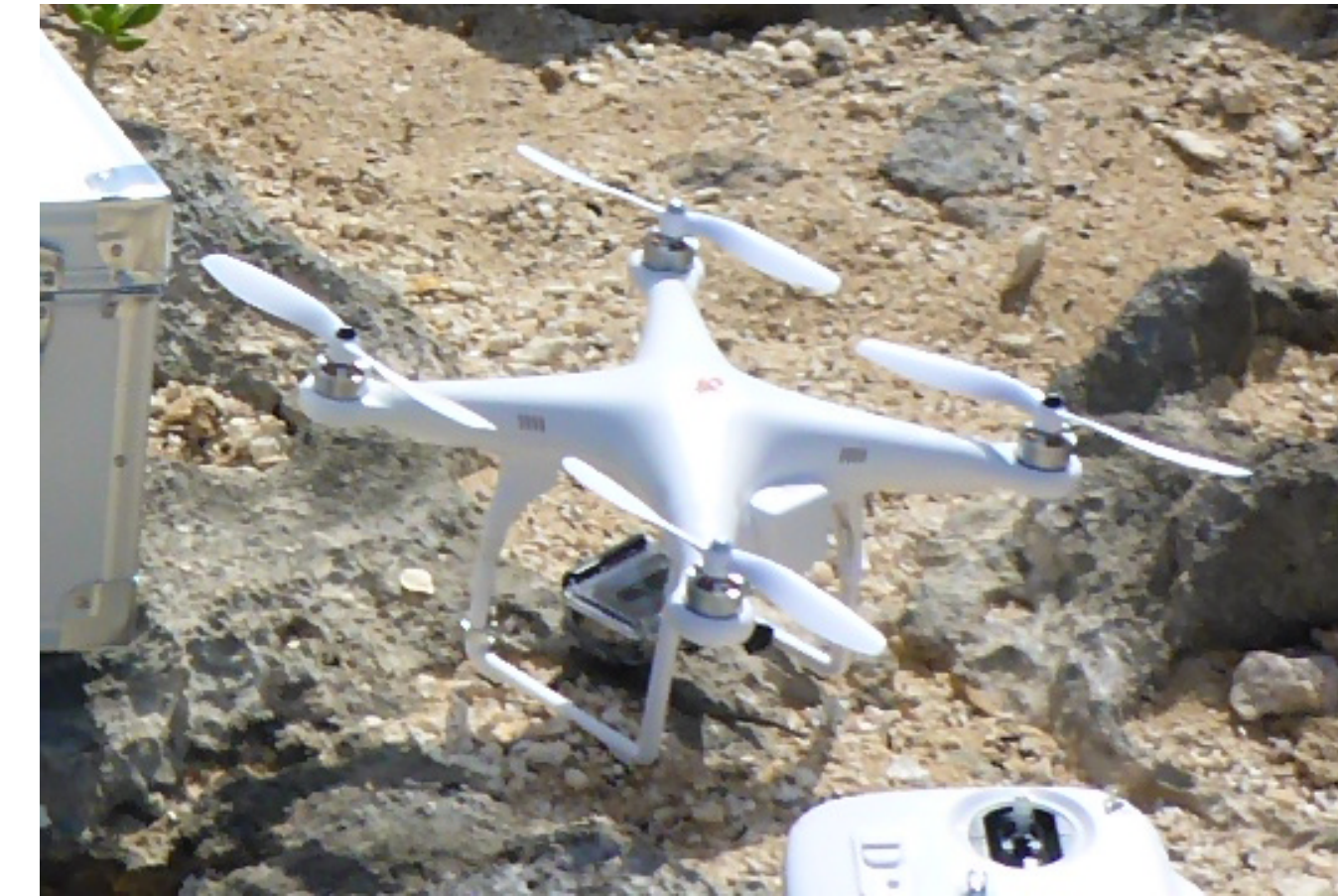
Figure 4: A DJI Phantom II UAV with a GoPro camera attached.
