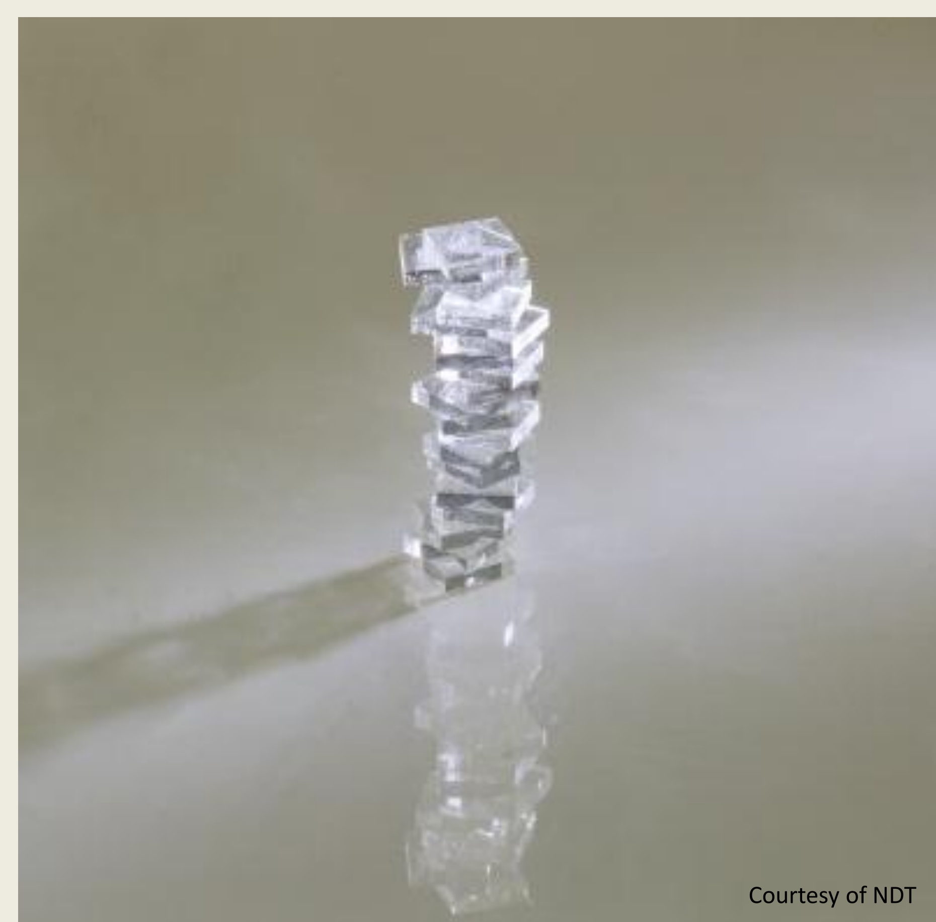
20 HPHT synthetic diamond plates from NDT, approximately 5x5mm square were studied and mapped. The [Si-V] defect was detected in 3 of the samples.
