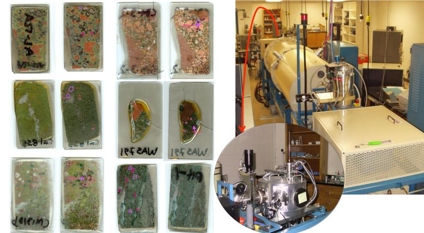
Figure 2 (left): The six sample slide maps, front and back, with sample sites of interest marked. Figure 3 (right): The HIBAL accelerator lab. The foreground shows the source oven and chamber. Subset image is the RBS chamber at the end of the line where samples are loaded.
