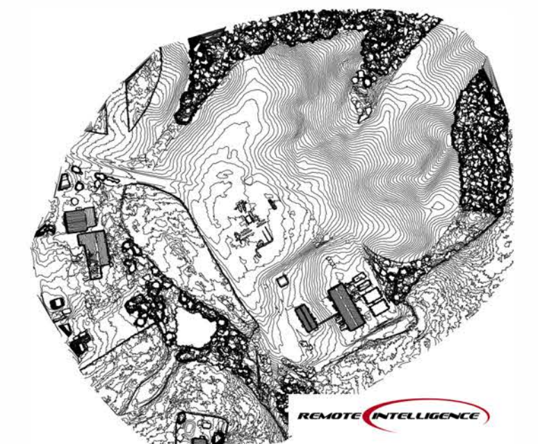
3D topographical contour line mapping application derived from systematic overlapping imaging of the subject area using UAV hardware and software applications.
