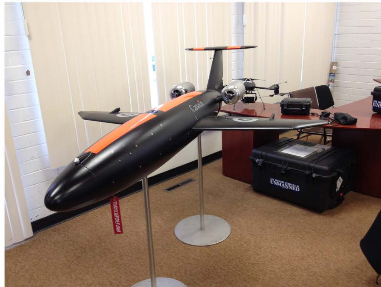
UAV utilized by Meggitt, a Canadian company based in Medicine Hat, Alberta, Canada which is closely connected with military and high-end UAV applications. This twin turbine powered UAV is intended to be flown beyond visual line-of-sight (BVLOS) at very high speeds.
