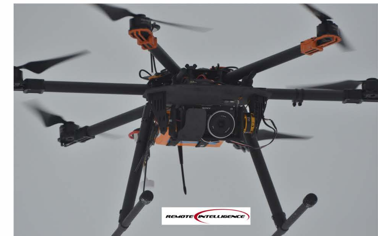
Highly sophisticated hexacopter used as an aerial photographing platform for image acquisition. Multiple, overlapping images using these costly platforms provides the basis for sophisticated mapping applications.
