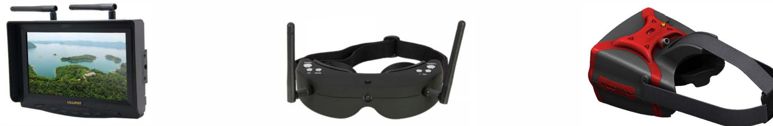
First person View (FPV) devices commonly used for monitoring mission flights. These aids provide valuable information for flight precision when used with additional input. Recording monitors provide a record of on-board systems checks of the UAV craft.
