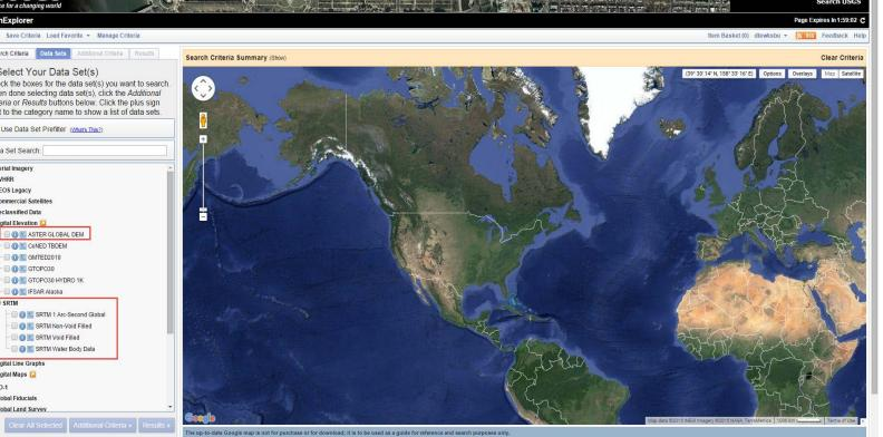
ASTER and new SRTM have the same resolution, 30 meters/pixel. The ASTER data was derived from stereo images so there are issues with areas that are routinely cloudy. The ASTER data covers higher latitudes than the SRTM data due to different orbital inclinations of the Space Shuttle and the TERRA satellite which carries the ASTER instrument. In the SRTM data group there are two listings for SRTM data. There is the 1 arc-second global and the SRTM void filled, which is the
