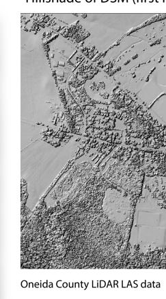
ArcMap hillshade of fir return data above. SD print of first return LiDA data (DSM), right. ? meter/pixel resolution X dimension 200 mm
