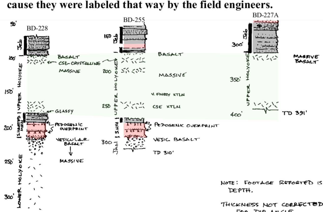
Upper Holyoke Basalt (pale-green) recovered in boreholes BD-228, BD-255, and BD-227A. It is 25.6 m (84') thick in BD-228 which is closer to the Cedar Mountain fault zone, and 29.1 m
