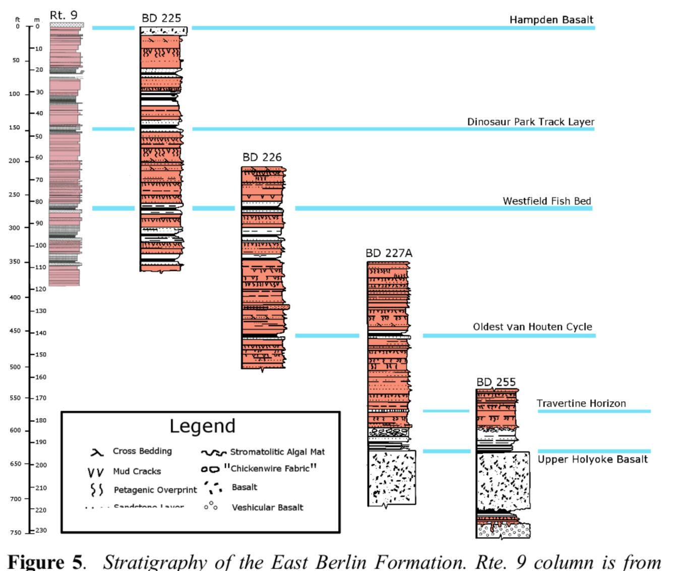
Olsen et al. (2005). BD-225 recovered core of almost the same stratigraphic interval, penetrating the 6 youngest van Houten cycles. "Westfield fish bed" is used as a correlation horizon to BD-226, which penetrated an older van Houten cycle that is used to correlate with BD-227A. The top of the upper
