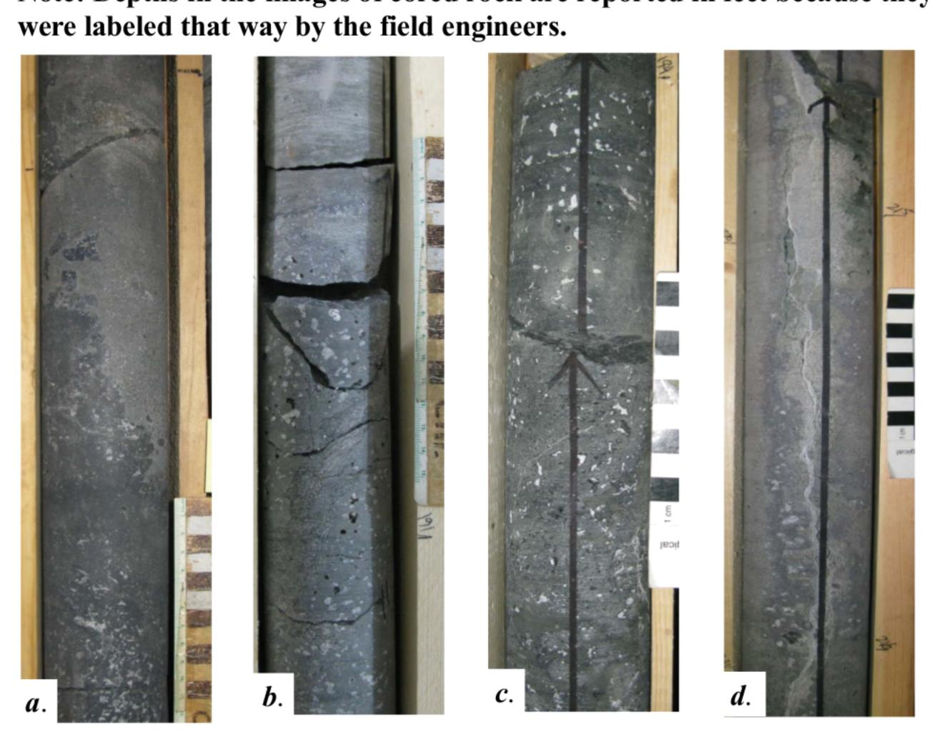
depth. Top of Hampden Basalt. c. BD-223, 193.8' depth. Upper part of Hampden Basalt ~2 ft (70 cm) below top. Note vesicular, brecciated, almost Scale in cm. d. BD-223, 215' depth. Fracture along which hydrothermal fluids altered the basalt. Sulfide minerals locally line the wall of the fracture. This is the deepest occurrence of vesicles (amygdales) in this core. (24', ~8 m, below
