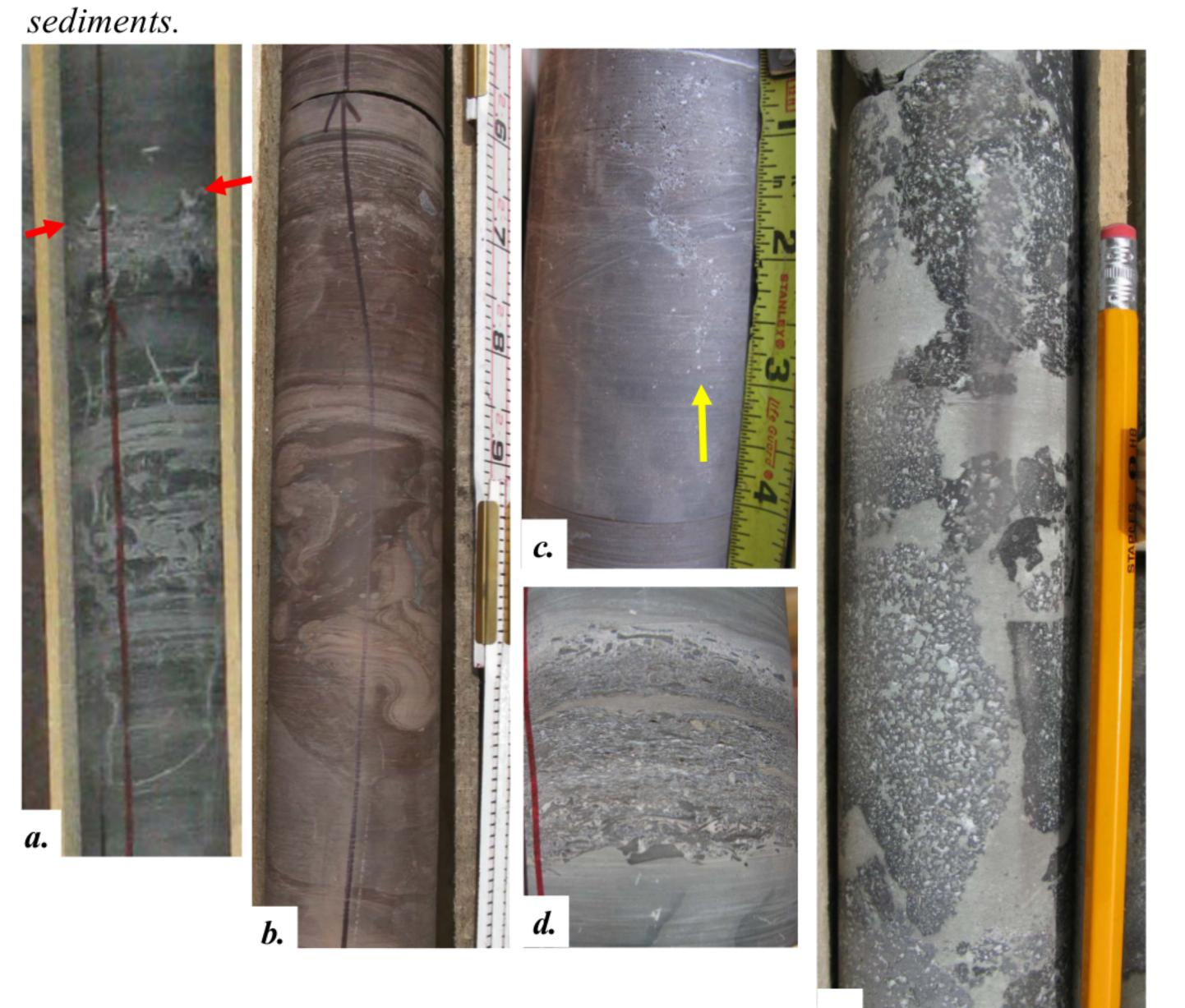
siltstone and very fine-grained sandstone. BD-255, 285+/-'; ruler calibrated i tenths and hundredths of a foot. c. Sandy siltstone with pedogenic overprint; trace of former sand-filled mud-crack (vellow arrow) in center. BD-228, scale in inches. d. Mixed siliciclastic/carbonate breccia in shoreline/shallow lake facies (see Fig. 10c). BD-255, 274', width of view 5 cm. e. Basalt-clast conglomerate above lower Holyoke Basalt. BD-228, 294' pencil for scale (width = 7 mm). References
