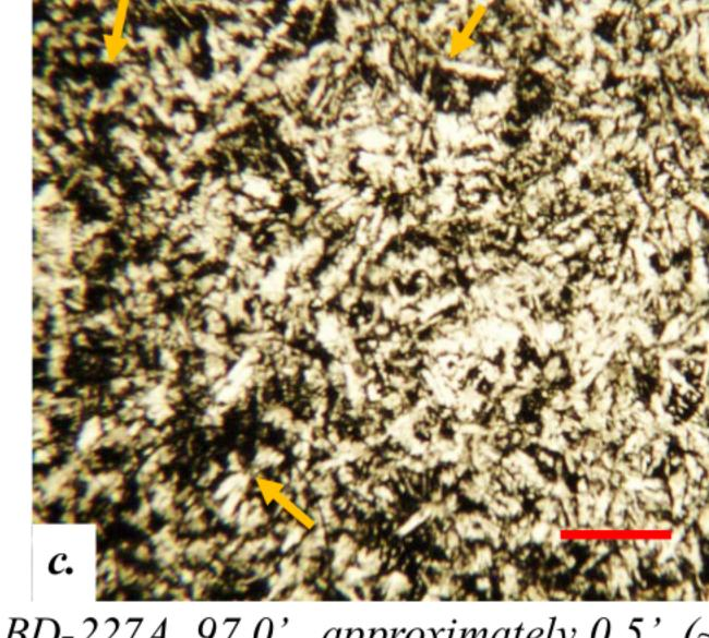
graph = 0.5 mm; all in plane light. a. BD-227A, 97.0', approximately 0.5' (~15 cm) below top of basalt; b. BD-255, 173.3', approximately 0.2' (~6 cm) below top of basalt; c. BD-227A, 97.1', approximately 0.6' (~18 cm) below top of basalt.
