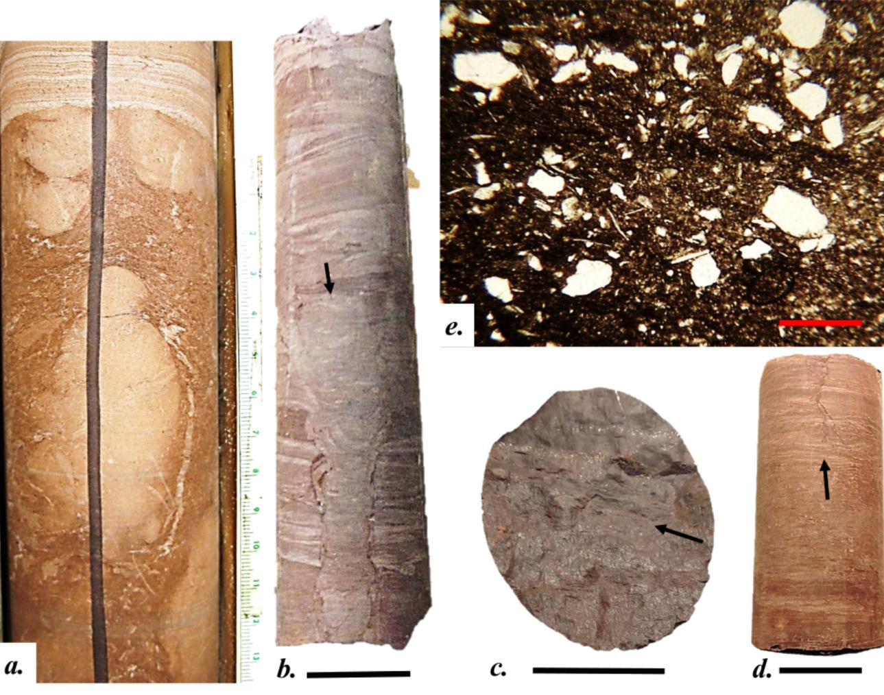
nodules in paleosol overlain by sheetflood deposit. Scale (on right) in cm. b. Sediment-filled desiccation crack (arrow), scale bar = 4 cm. c. Slickensides (arrow), scale bar = 4 cm. **d**. Root trace (?) above arrow, scale bar=4 cm. **e**. Thin section micrograph showing disruption of bedding and bioturbated (?) fabric, plane light, scale bar = 0.5 mm.
