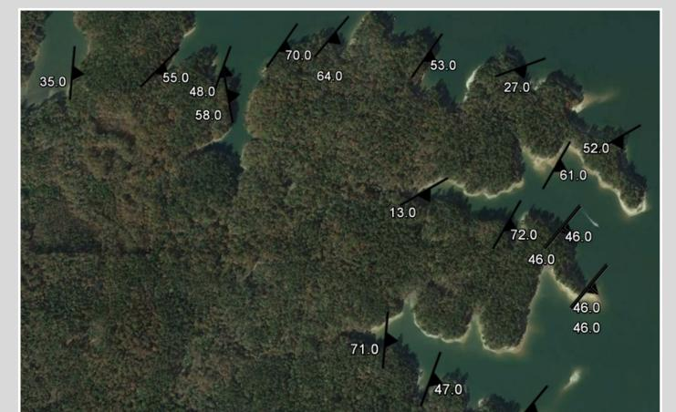
Figure 11. Custom placemarks, such as these strike and dip symbols, can be created from any raster image and bulk inserted from an Excel spreadsheet. By incorporating azimuth information, structural symbols can be rotated into their prop er orientation.
