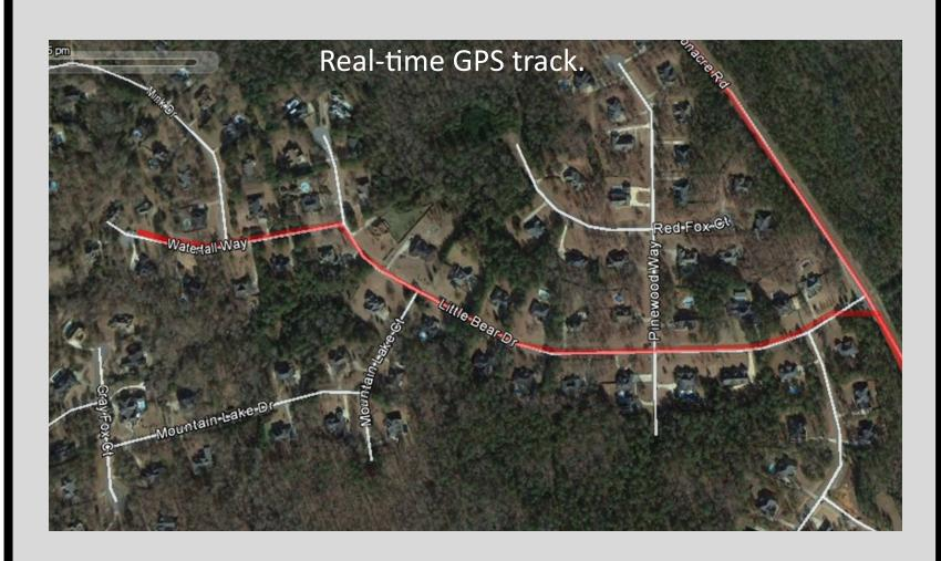
Figure 4. Recent aerial imagery, roads, and a linked GPS allow for instant determination of location and real-time correction of low resolution GPS data.
