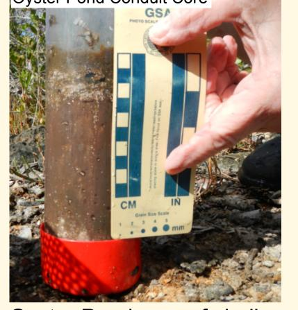
reddish-brown mud. capped by coarse, lightall overlain by thick floc layer. grains, capped by floc Other parts of Oyster Pond and whole gastro ntained only floc over bed- pods.
