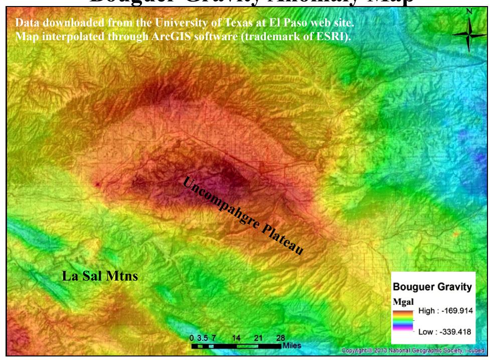
Figure 10. Bouguer Gravity map of the La Sal Mountains and part of the northwestern Uncompany Plateau shows areas of gravity highs (>-150 Mgal). These anomalies are likely to be related to high density rocks at depth, possibly mafic types. in the crust (see Fig. 11 below).
