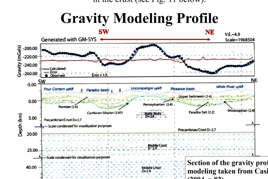
Figure 11. Casillas (2004) creates the geometry of the possible existence of the mafic body in the Uncompany Plateau. His result shows the calculated and observered gravity anomalies are nearly compatable for the mafic body with the assummed density of 2.83 gm/cm<sup>3</sup> at  $\sim$ 5 KM depth.
