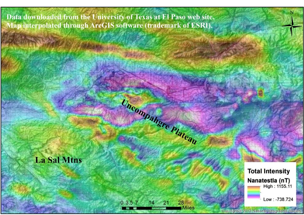
Figure 9. The aerial residual magnetic map shows strong anomalies in the La Sal Mountains and central part of the northwestern Uncompany Plateau. These magnetic anomalies indicate magnetic sources in the crust.
