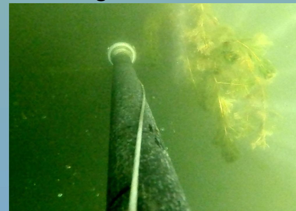
Fig 3. Piston corer attached to rods lowering into the south basin.
