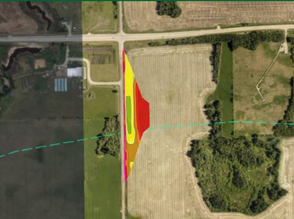
Fig 5. Superimposed Edgemont ERT cross section over a buried valley boundary that can be identified in profile.
