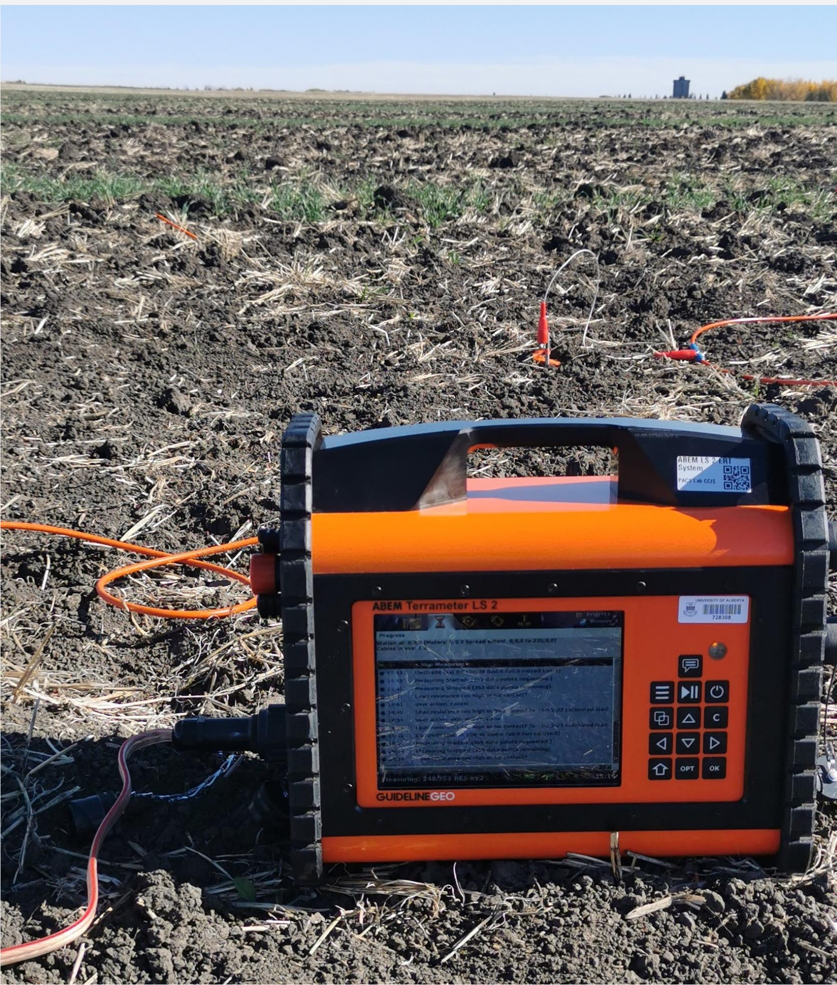
Fig 2. ABEM ERT System and attached cables at the UofA Farm site.
