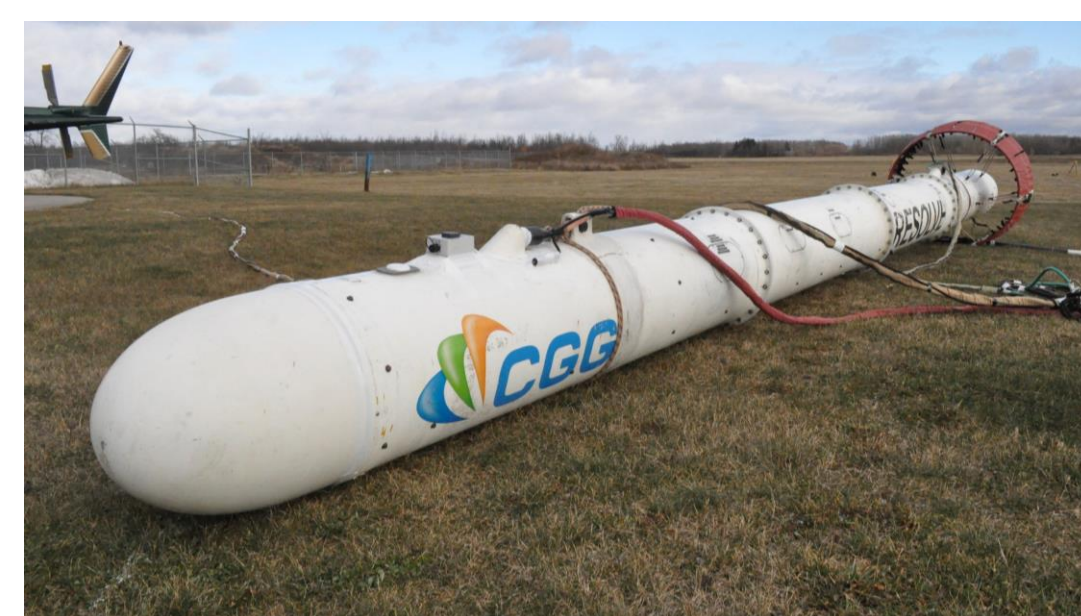
An airborne frequency-domain and residual magnetic survey was completed over the study area using the RESOLVE™ system shown here. The RESOLVE™ "bird" is 9 m long.
