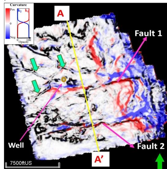
Figure 6a. Most positive principal (k1) and most negative principal curvature(k2) attributes co-rendered with the Sobel filter similarity along the Detrital surface. This figure allows visibility of the fault throws (blue- downthrown, red- upthrown) and edges of features (black). The green arrows show the possible channels.
