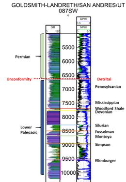
Figure 2a. Digital log showing the gamma ray, density porosity and neutron porosity logs highlighting the various formations and the Pennsylvanian unconformity as seen by the well.
