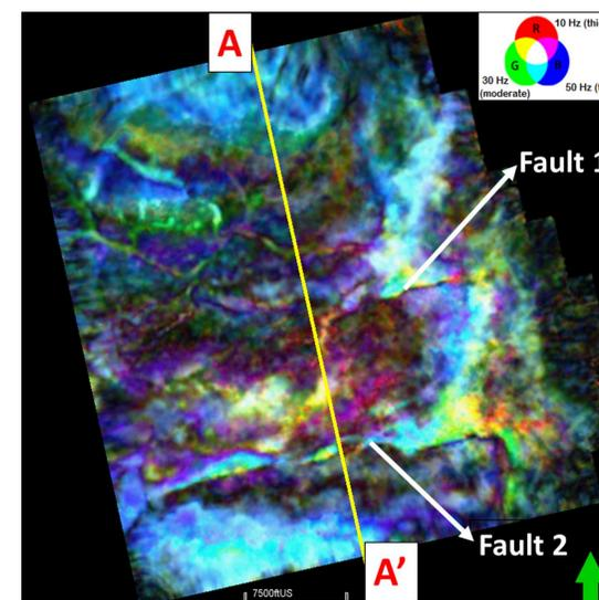
Figure 6b. RGB blending of the spectrally decomposed volumes at 10Hz, 30Hz and 50Hz frequencies along time slice at 1090ms (very close to the detrital surface) highlighting the faults, thickness of beds and variation in lithology. Note the NW-SE oriented channels in the north central part.
