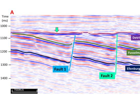
Figure 4. Seismic crossline 5130 showing the two major faults and the Detrital, Fusselman and Ellenburger horizons (Modified from Szyplski, 2021). The green arrow shows the probable channel.
