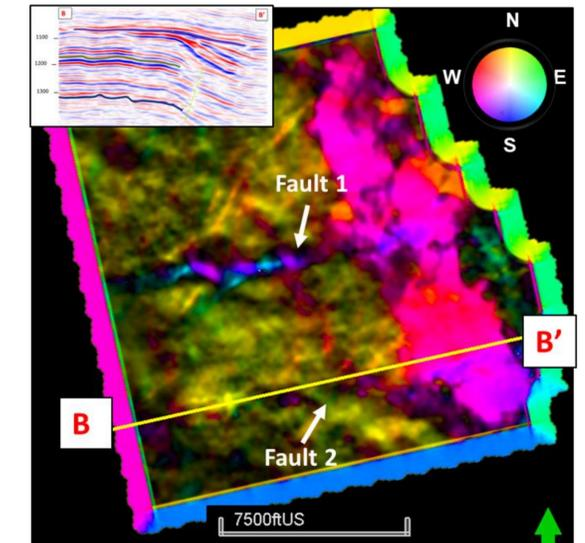
Figure 6c displays the reflector convergence attribute highlighting both faults and the pinch-out direction of the angular unconformity.
