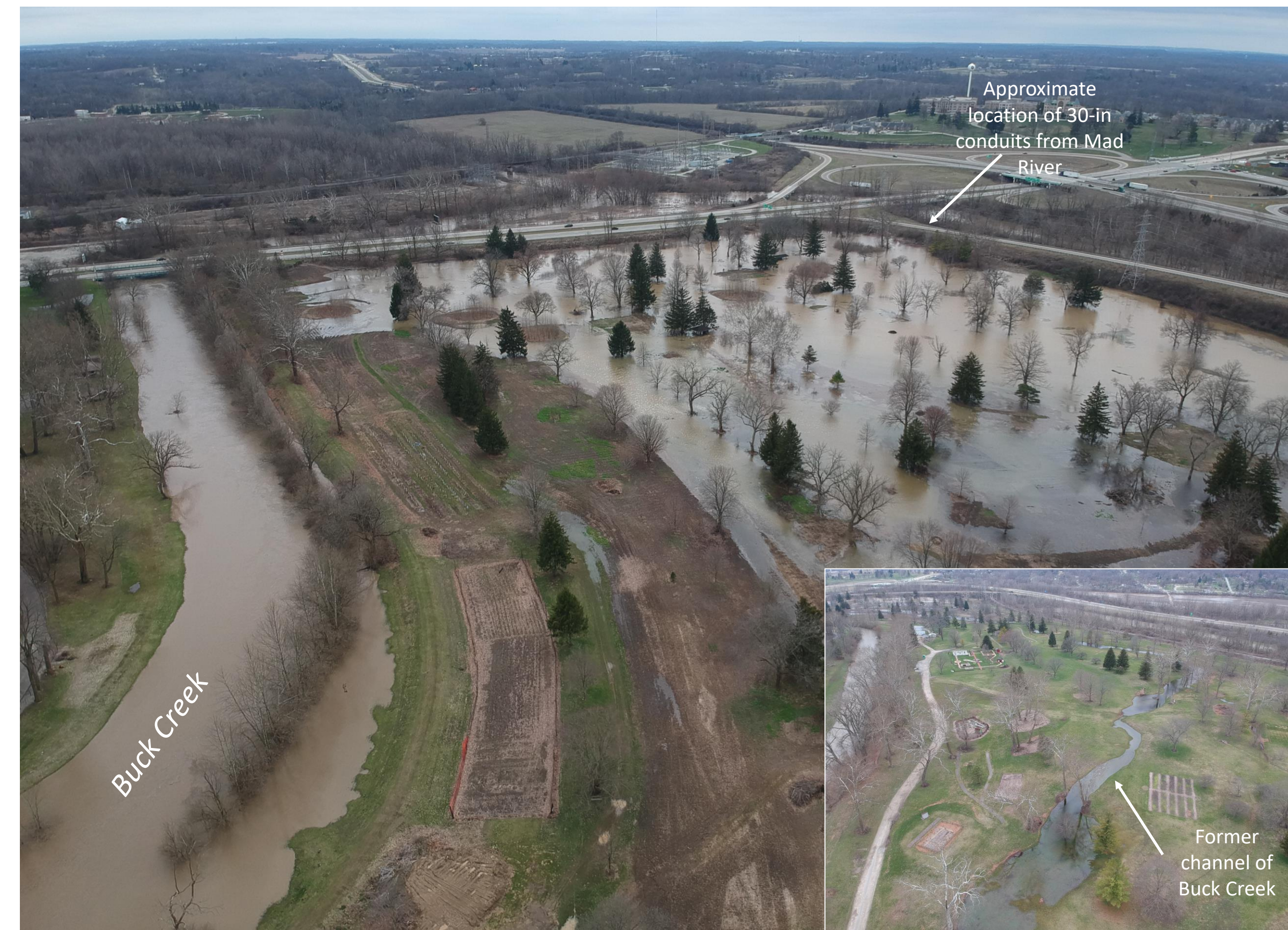
Figure 4. Flooding in March 2020 covered approximately 18 ac of the former SPGC. Buck Creek is separated from the course by a levee. Though flooding occurs when Buck Creek is high because of permeable sand and gravel outwash underlying the levee, extensive flooding such as shown here occurs through two 30-inch conduits connecting SPGC to the Mad River. During exceptionally high flow, flooding extends further onto the former SPGC along abandoned channels of Buck Creek from the time of channelization (inset).
