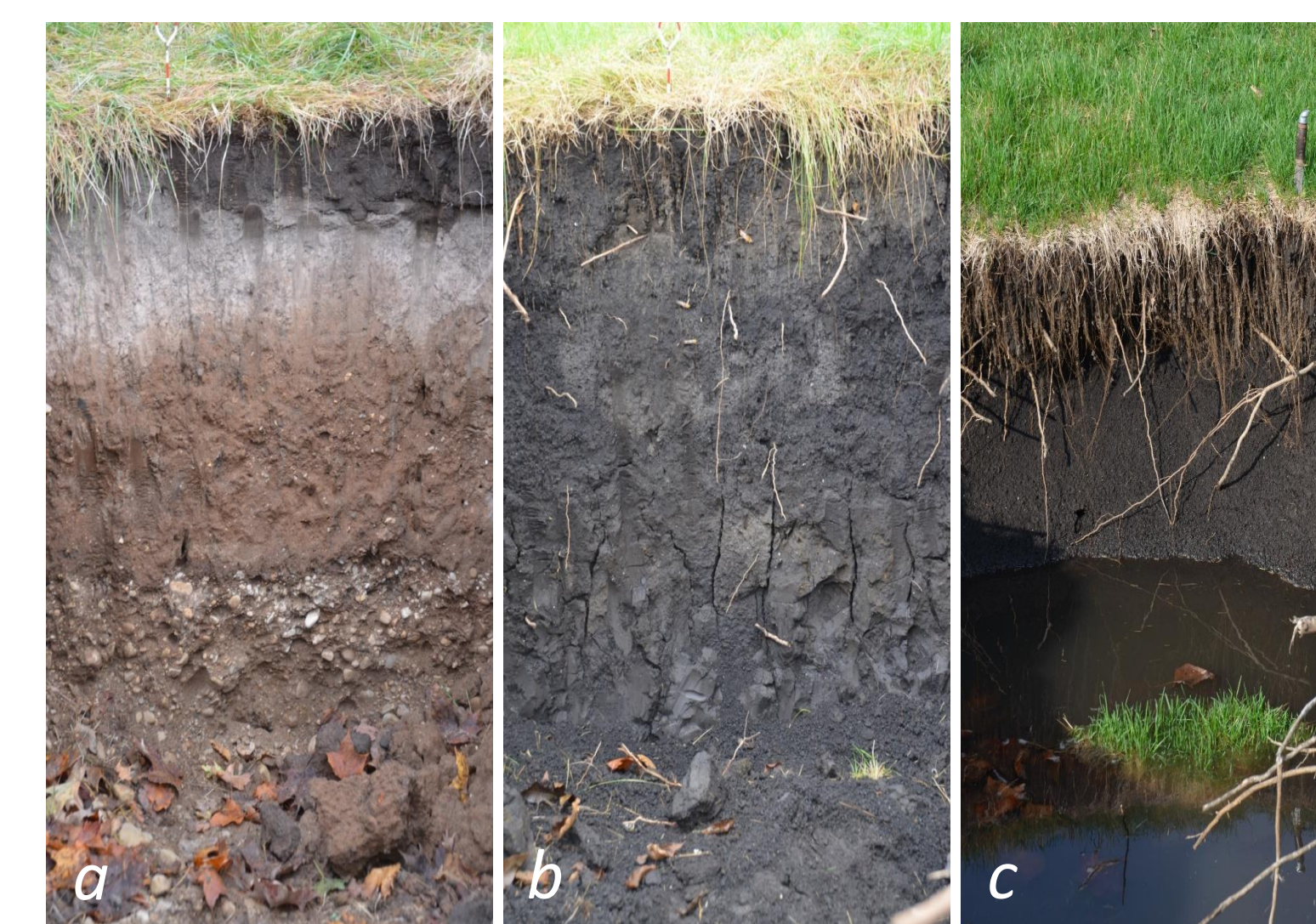
Figure 10. Two soils are present on the former SPGC, (a) Eldean and (b) Westland soil series. The Westland is classified as a hydric soil in Ohio and comprises more than 98 percent of the former course. The sand and gravel that form the parent material for the Eldean (a) underlie the entire area and form a highly-productive buried valley aquifer. (c) Because of the high hydraulic conductivity of the sand and gravel, while lower elevations of Westland soils are inundated, the water table in dry areas rises nearer the surface on Westland soils at higher elevations. Excavation of the upper part of the Westland soil would enhance storage potential and, in lower areas, restore it to its natural condition as a riparian wetland.
