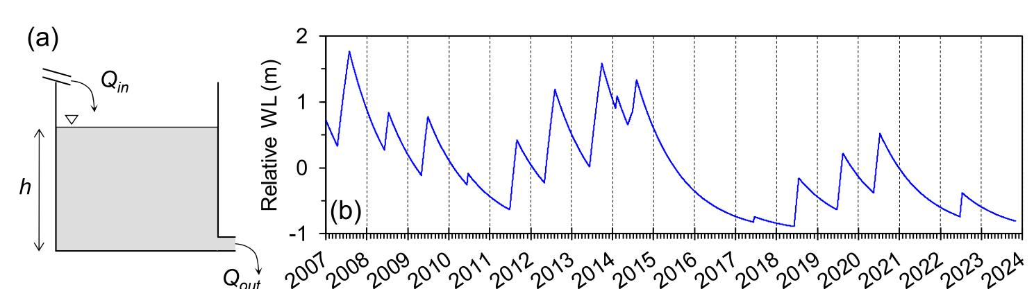
**Fig. 7** (a) Simple linear-reservoir model representing the watershed-scale aquifer storage, consisting of recharge input  $(Q_{in})$ , discharge output  $(Q_{out})$ , and water level (h). (b) Response of the linear-reservoir aquifer response to interannual variability in recharge simulated by VSMB.
