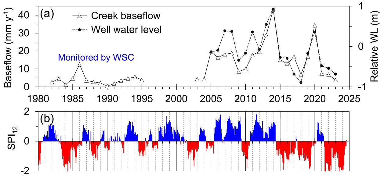
Fig. 8 (a) West Nose Creek (WNC) baseflow and the average water level WNC monitoring wells in October of each year. (b) Standard precipitation index (SPI) in Calgary, calculated with a 12month leading period. Flow was monitored by the Water Survey of Canada (WSC) at the same location during 1982-1995 until the station was discontinued.
