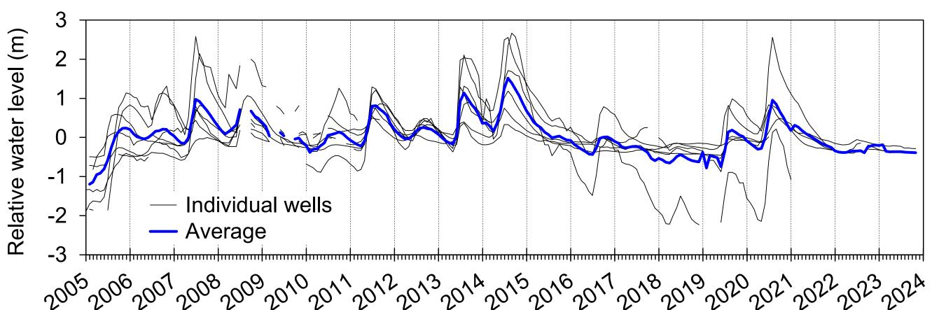
Fig. 6 Water levels in the WNC monitoring wells (see Fig. 1 for locations). Values are relative with respect to the long-term mean of each well. The thick line indicates the average of all wells with available data. Major tick marks on the horizontal axis indicate January 1.
