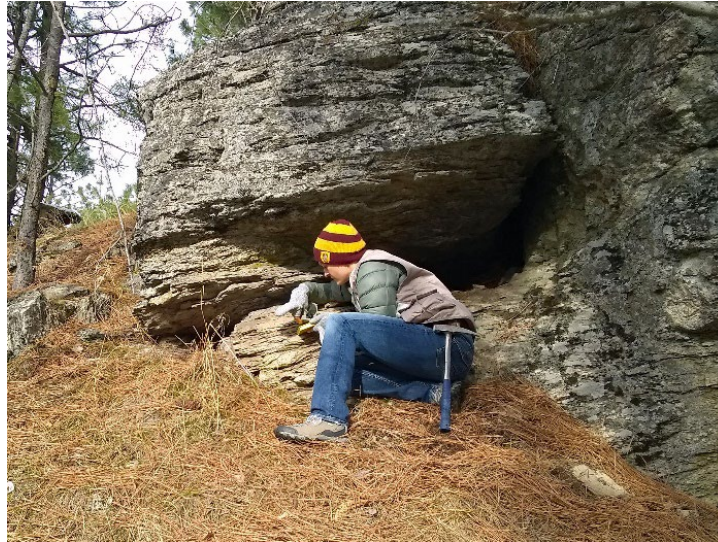
Figure 3. Taking strike and dip measurements using a Brunton compass.
