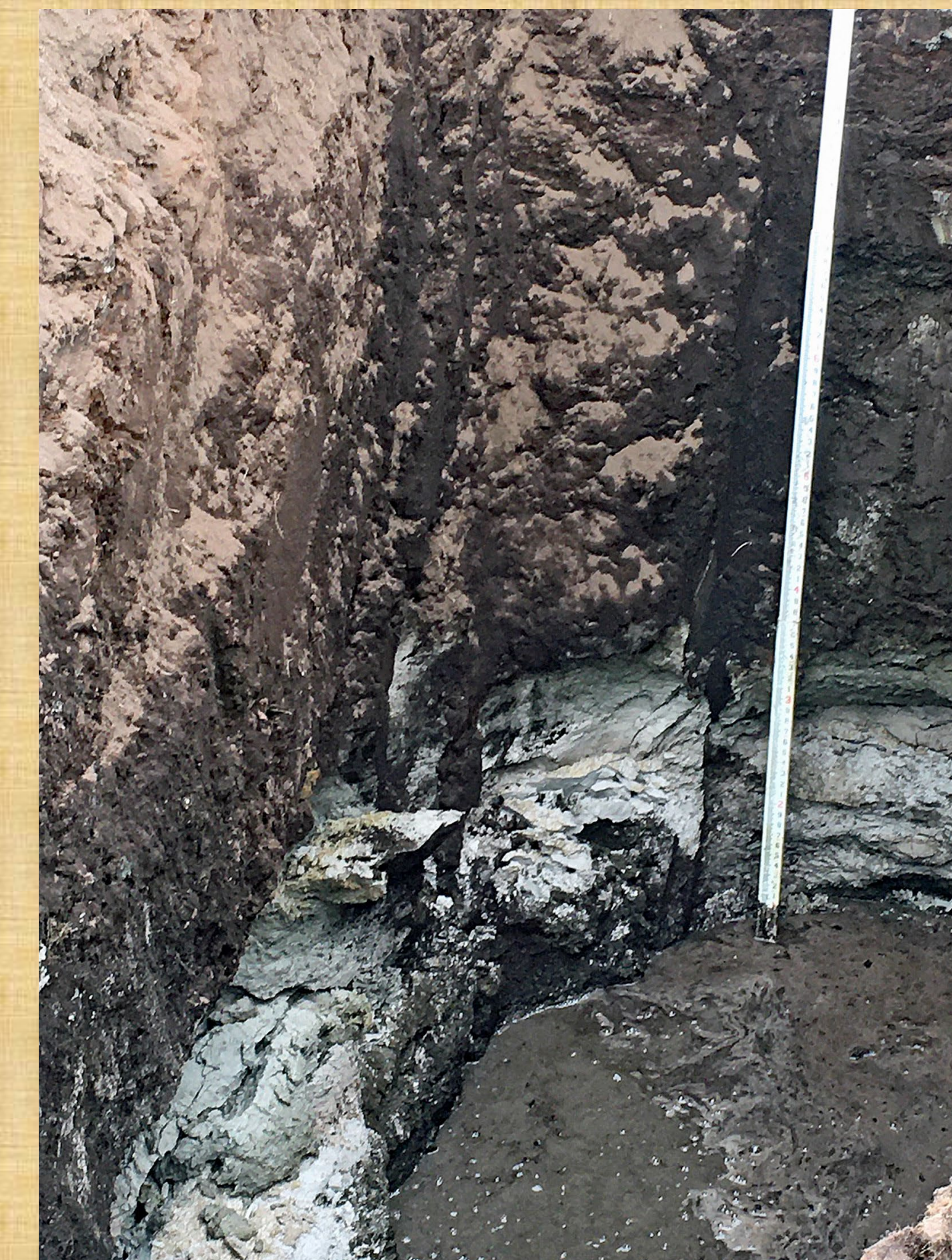
Stratigraphic column of Saltese Flats trench with the ash samples indicated by SF-2U & SF-2L (left). Measurement of stratigraphic relations using a stadia rod (center). Close-up of ash layer showing sharp upper contact with peat; sharp lower ash contact not shown due to rapid groundwater inflow (right).
